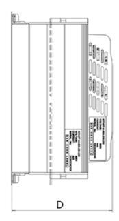
Control voltage (terminal A1, A2) = 230AC D = 305 Digital control voltage (terminal 1-5) = 24DC H = 791 Kg = 54 W = 510
